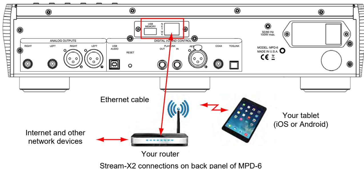
**Streamer Network:** Connect this to your network router and make sure it is connected to the internet and its wireless network is active. The Stream-X2 needs this network connection to connect and play any streaming media from the internet. It also uses it to connect to your tablet for remote control or to your Roon server.
