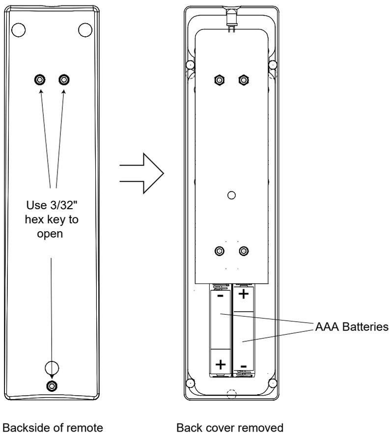
The remote operates with 2 AAA size batteries. In order to change them the back cover needs to be removed as shown in picture on the left. Make sure that replacement batteries are inserted with their polarities as indicated in the picture. The screws can be opened with a hex 3/32 inch key.
