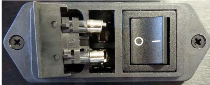
4. Replace both fuses with 1.6A / 250V slow blow types. Length is 20mm
