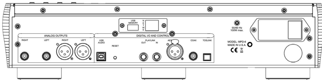
**Digital outputs:**      **PLAYLINK OUT:** Proprietary optical link to other Playback Designs equipment. This connection supports multiple audio formats natively for PCM and DSD.
