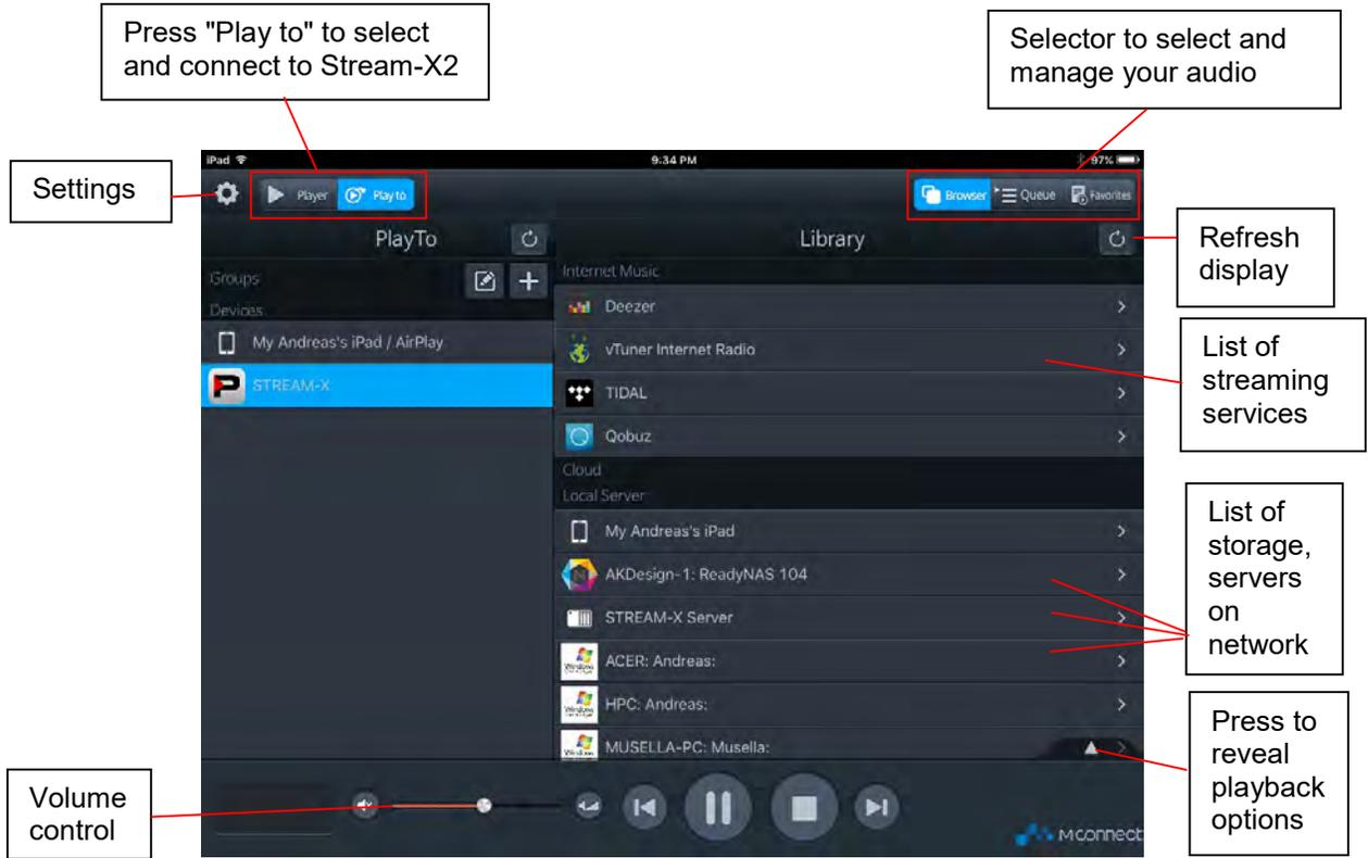
6. If you launched the app for the first time it is possible that Stream-X2 is not yet connected to the app. Just press the button in top left corner "Play to" and select Stream-X2 from the list that appears below.
