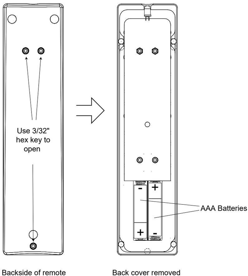
The remote operates with 2 AAA size batteries. In order to change them the back cover needs to be removed as shown in picture on the left. Make sure that replacement batteries are inserted with their polarities as indicated in the picture. The screws can be opened with a Philips screw driver.
