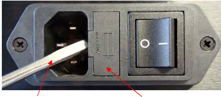
Prying open with small screw driver
