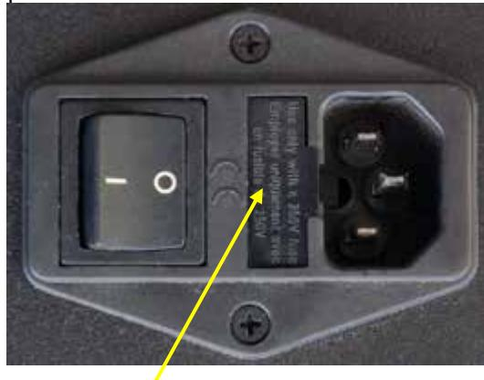
2. Use a small screw driver to pry open the fuse holder.
