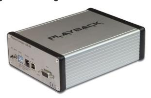
The USB-XIII is a 3rd generation USB interface designed to operate in conjunction with Playback Designs' 3- and 5-series players and DAC's. Its capabilities have also been expanded to work with any other DAC equipped with either a AES or Coax input.
